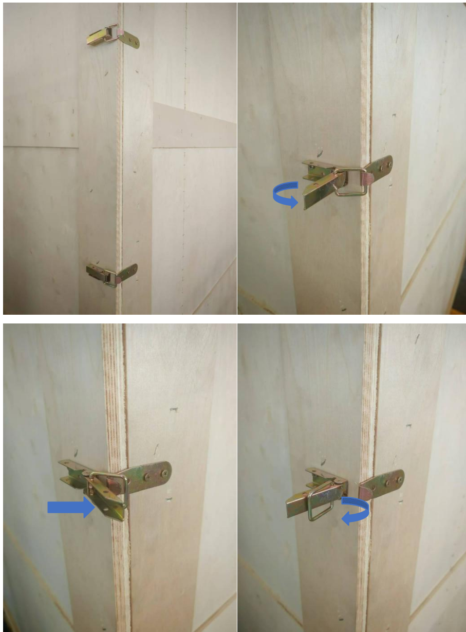
Figure 5.1.1 Schematic diagram of wooden box fixing buckle operation
