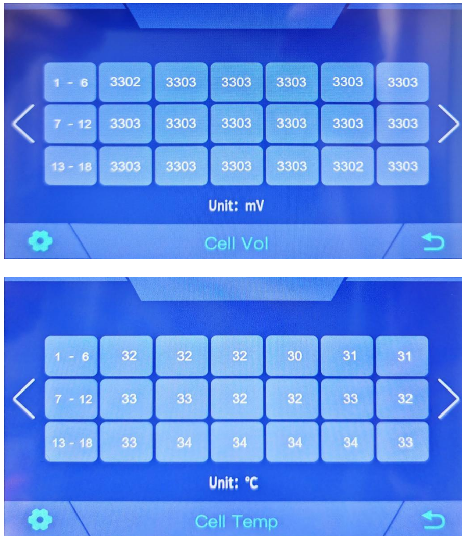
Figure 2.4.6 HMI Individual Information View
