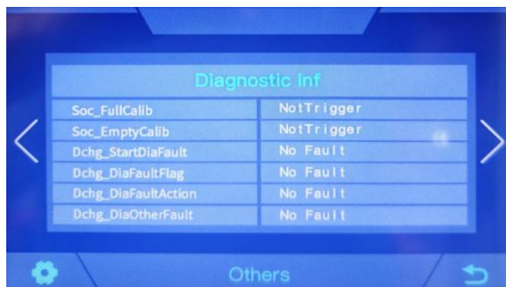
Figure 3.5.5.2 Battery fault information interface
