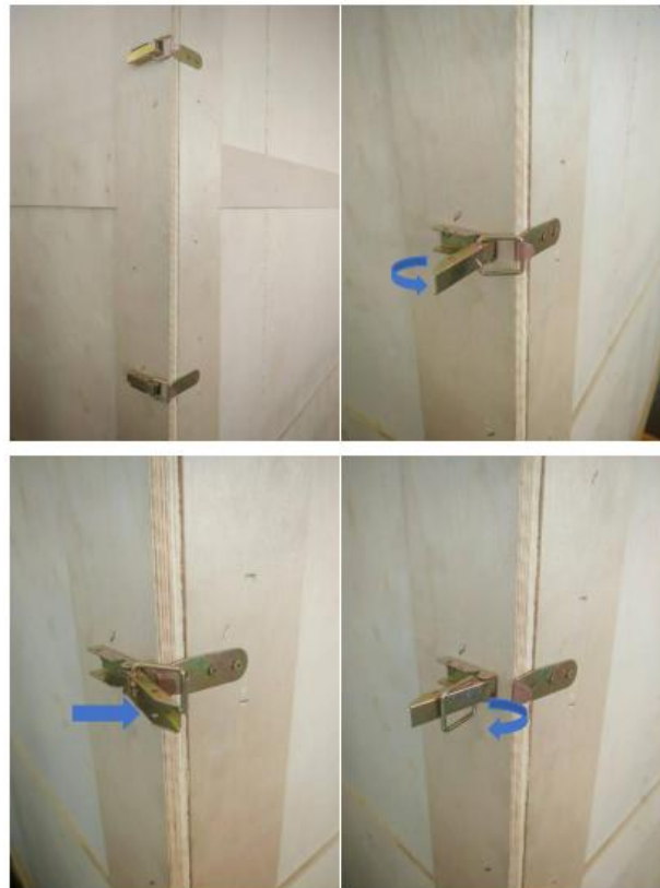
Figure 6.1.1.1 Instructions for securing the wooden crate
