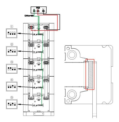
If the bottom of the last battery's connecting copper bar appears to be suspended, install the copper bar gasket that comes with the package underneath the copper
