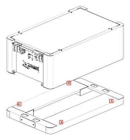
Step 3 Align with the locating pins on the base and stack the battery onto the base
