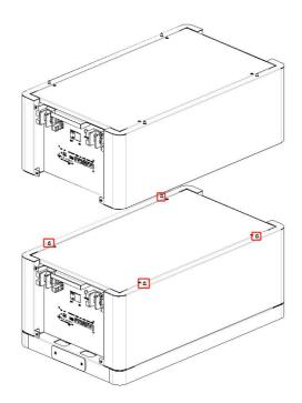
Step 4 Align with the locating pins on the battery, stack another battery onto the previous one, ensuring the orientation is consistent, and repeat the process up to a maximum of 5 layers
