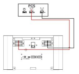
Step 1 Connect the battery DC+ to the inverter DC+/BAT+
