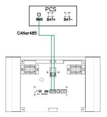
Step 1 Insert one end of the RJ45 communication line into the communication interface (CAN or RS485) of the battery host inverter
