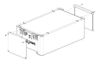
Step 6 Install the side panels back to the battery
