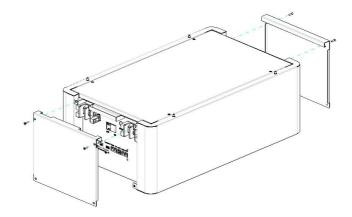
Step 2 Remove the side panels on both sides of the battery
