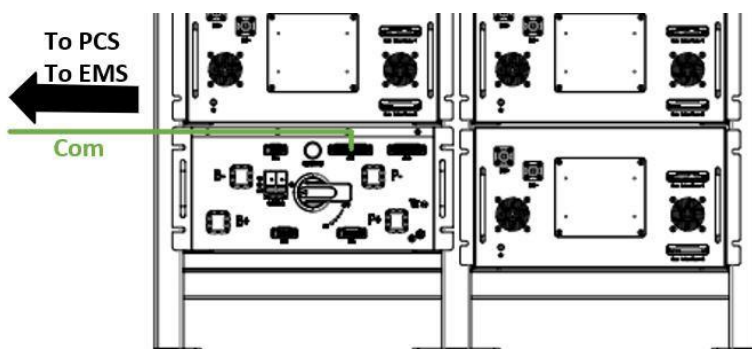
Figure Schematic diagram of battery cluster external communication cable installation
