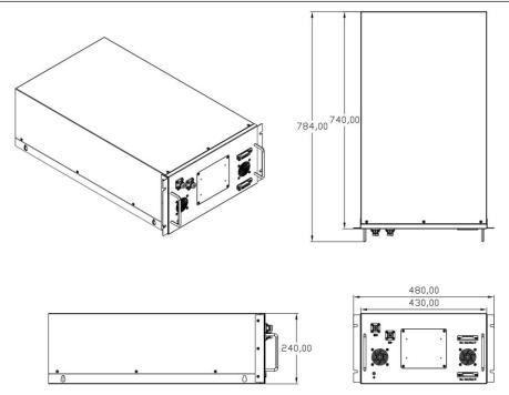
Figure 3-view of battery pack dimensions
