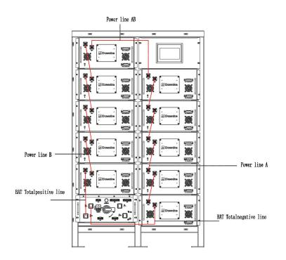
Figure Schematic diagram of battery cluster electrical cable installation
