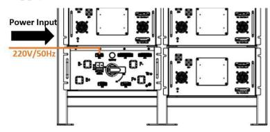
Figure Schematic diagram of battery cluster external power supply cable installation
