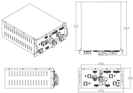
Figure Dimension of high-voltage cluster control box
