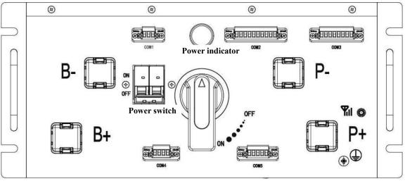
Figure Panel of high-voltage cluster control box
