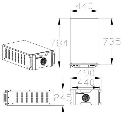
Figure 3-view of battery pack dimensions
