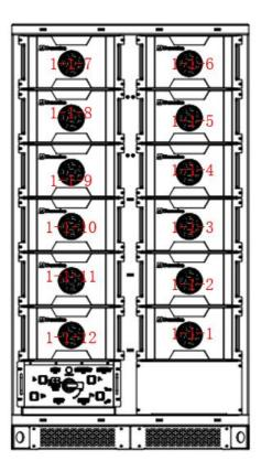
Figure 1. Battery pack installation sequence diagram
