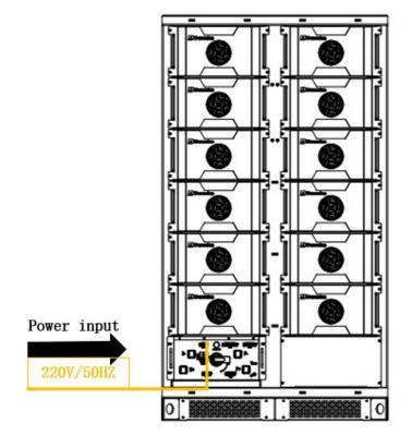
Figure Schematic diagram of battery cluster external power supply cable installation
