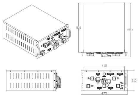
Figure Dimension of high-voltage cluster control box
