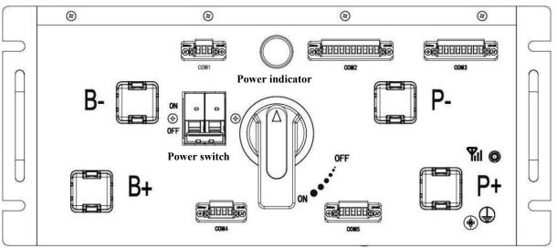
Figure Panel of high-voltage cluster control box
