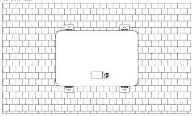
Step 2: Hold the wall-mounted battery against the wall to ensure that it is placed securely, use a marker to mark the location of the hole punched, and set aside the battery.
