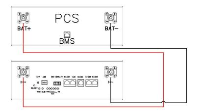
Step 1 Connect the battery DC+ to the inverter DC+/BAT+ Step 2 Connect the battery DC- to the inverter DC-/BAT-
