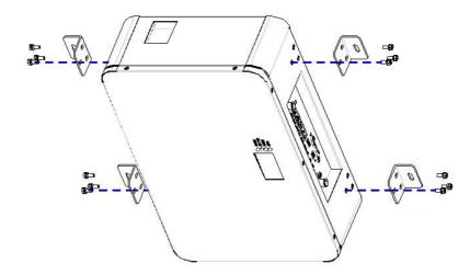
Step 1: Install the mounting ears onto the battery as shown in the diagram, with a torque of 10 N.m.
