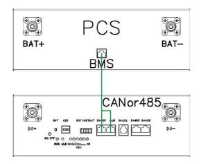
Step 1 Insert one end of the RJ45 communication line into the communication interface (CAN or RS485) of the battery host inverter
